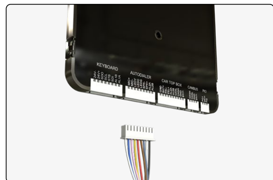
Cable has 9 terminals and plugged in AUTODIALER connector in MEGA7 series as shown.
